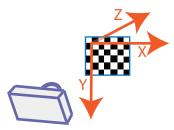
When you reconstruct a 3-D scene from multiple views containing a calibration pattern, the resulting 3-D points are defined in the pattern-based coordinate system. The "Stereo Calibration and Scene Reconstruction" example shows how to reconstruct a 3-D scene from a pair of 2-D images containing a checkerboard pattern.
